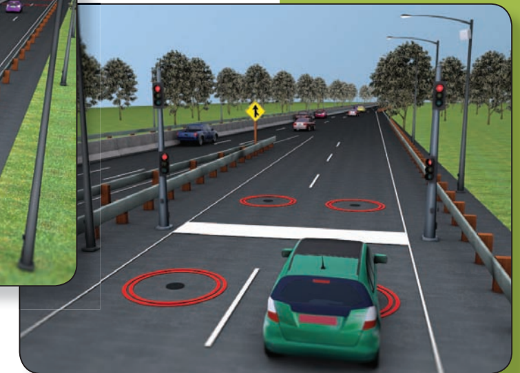
ADAPTIVE RAMP METERING
